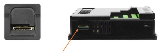
Figure 9.1 – Removable microSD Memory Card Slot
