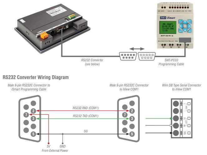
The 5V external power can be supplied from USB port or external 5V power supply. The USB port in the iView has 5V output which can be used to power-up.
