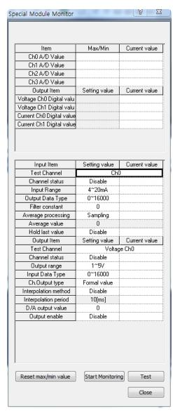
(4) Start Monitoring: Click [Start Monitoring] to show digital input / output data of current operated channel.
