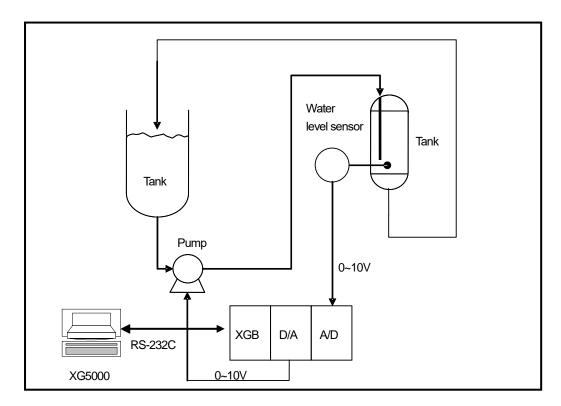
[Figure 6.17 Example of water level control system]
