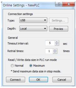
(c) After choosing the connection method with the PLC to be deleted, if you click <code>"Access\_"</code> or <code>"OK\_"</code>, all PLC programs, parameters, data, passwords will be deleted.
