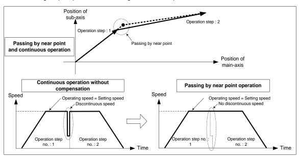
In the picture above, during general Continuous Operation, Occurring speed discontinuity because of remaining amount of movement at the last operation step NO.1. 「Near Passing」 Continuous Operation, you can move the remaining amount of movement to next step and execute Continuous Operation without speed discontinuity.
