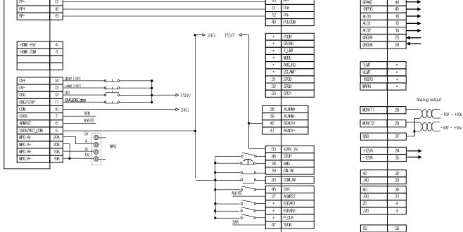
Note 1) Input signals DI1 to DIA and output signals DO1 to DO5 are default signals allocated by the factory.
