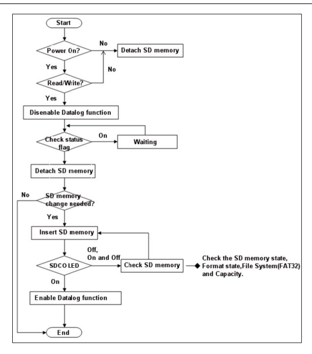
2) Power off or reset during data log run may cause abnormal data saving. Also, the file system may be damaged and not recognized the SD memory and the files. In cases of power off during data saving, the SD memory diagnosis function is activated, and other PLC functions are not performed during that time (approximately 15 seconds).
