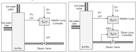
[Figure 15.13 Comparison of single loop control and cascade control]
