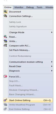
(3) Then, the background color of the program window changes and it is converted into the mode of modification during RUN.
