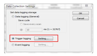
4) Upon selection, the following window is activated for trigger setting. Select [Multiple Condition] as Trigger Condition, Select either [Elevation] or [Descent] as the Trigger Occurrence Condition.
