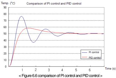
(d) Considering table 6.5, in case PID control is used, max. overshoot decreases from 16.5°C to 8.5°C. At this time, P coefficient, integral time, derivative time are not optimal values, just one of the examples. Actually, P coefficient, integral time, derivative time values vary according to PID control system.
