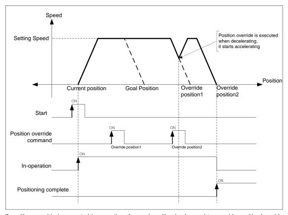
If position override is executed in operation, the goal position is changed to override position1 and keep operating. If position override for override position2 is executed at dec. area, positioning is finished by acc. speed already set at override position2.
