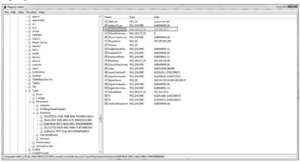
6) Click with the right mouse button on the right screen of the relevant folder and select New]→[DWORD(32bit) value].
