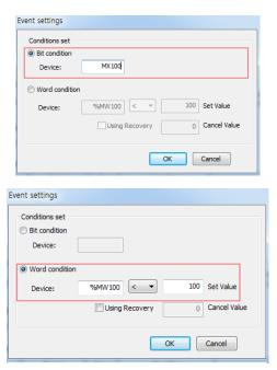
6) When setting is complete, the window closes and the conditions initially set at the Event Setting Condition menu are displayed as follows.
