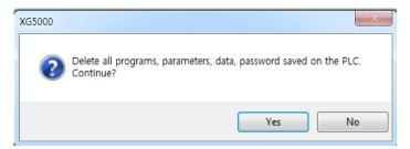
(b) If you choose "Yes" in the dialog box, the window for selecting the connection method with the PLC to be deleted is created.
