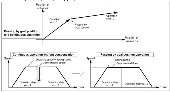
It decrease speed of acceleration, constant speed section as much as remaining amount of movement at the last section of current step to compensate position if operates as passing goal position operation.
