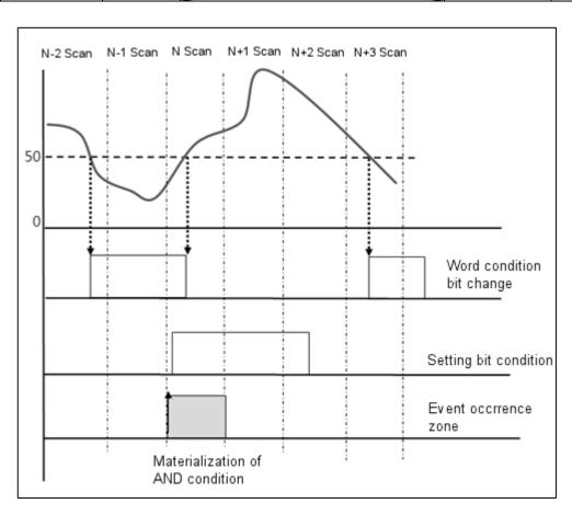
₩ When setting with combination of BIT and WORD conditions (release value set)
