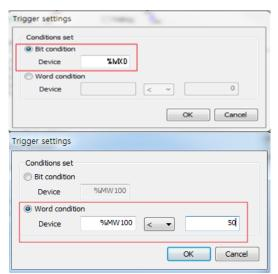
When setting is complete, the window closes and the conditions initially set at the Trigger Setting Condition menu are displayed as follows.
