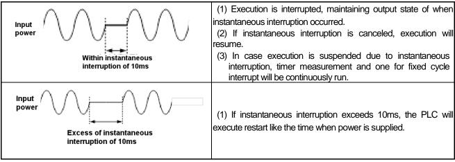
The below figure shows the PLC's execution processing flow chart when instantaneous interruption occurs.
