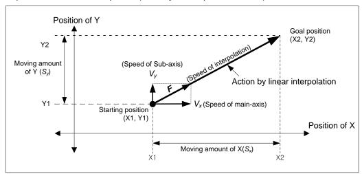
Interpolating speed(F) = Operating speed of main axis
