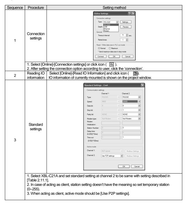
After standard settings, P2P channel and P2P block should be set. Setting methods are as follows.
