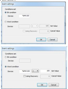
7) When setting is complete, the window closes and the conditions initially set at the Event Setting Condition menu are displayed as follows.
