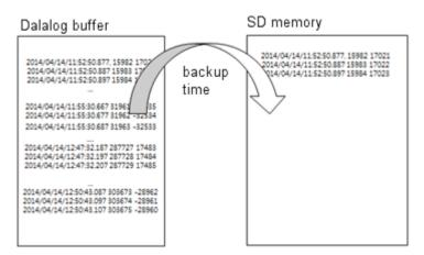
To prevent this, the collected data need to be saved into the data at certain intervals regardless of the storage. The data saved into the SD memory is not lost even in case of sudden power change. Backup time can be set at from 1 to 5 seconds. However, setting too short backup time may affect data log performance.
