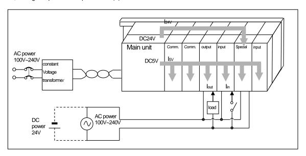
(e) Input average power consumption of input module (power consumption of simultaneous On point)
