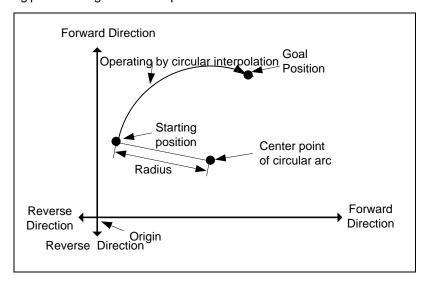
2) If the goal position is same as starting position, it is available to have an operation like a circle that has distance from starting point to auxiliary point as its radius
