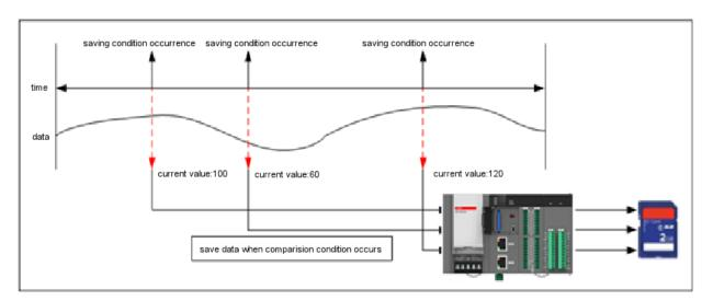
The collected data at each set cycle are scan END processed and saved into the SD memory as a CSV file.
