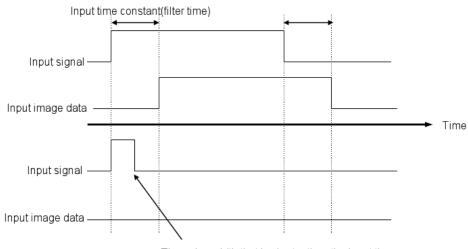
The pulse width that is shorter than the input time constant is not regarded as the input signal.
