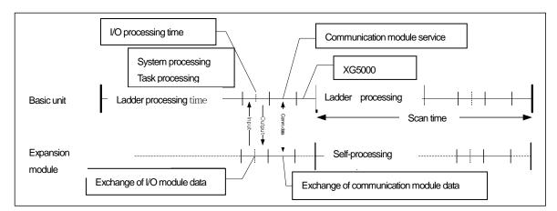
Scan time = Ladder running time + system processing time + digital module I/O processing time + analog I/O processing time + communication module processing time + XG5000 Service processing time
