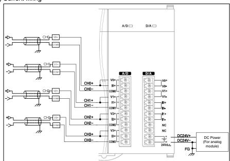
(6) The example of analog input 2-Wire sensor/transmitter wiring(The current input)
