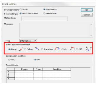
5) Select each condition setting menu one by one, inputting specific set values. [Multiple Condition] activates Event Condition by calculating [Single Conditions] using the set run method. The basic setting is performed in the same way as Single Condition.
