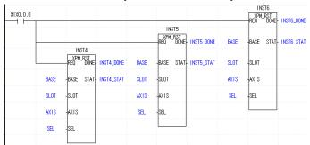
However, in the case of XPM\_VRD, you cannot simultaneously execute function blocks within a single scan not only for the same axes but also for different ones. If you execute the XPM\_VRD commands at the same time in one scan, the error code 811 will occur and XPM\_VRD will not work after the first XPM\_VRD.
