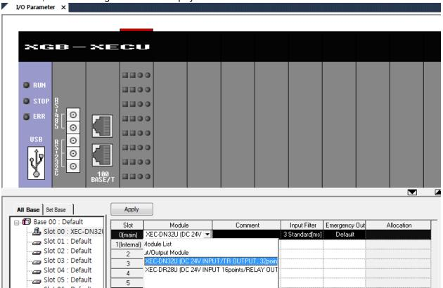
If you click the <code>"Module\_"</code> in the <code>"slot\_"</code> position, the list of each module will be displayed. Then, choose the module that is matched with the actual system to be configured. The selected slot will be displayed as below.
