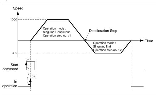
The Step1 will be operated by the start command. however, because the goal position of next step is on opposite direction from the goal position of step1, it stops after deceleration, and then operate Step2 to a opposite direction.
