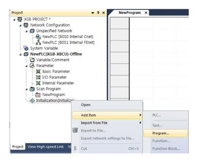
(d) Make the necessary initialization program and make sure to include the INIT\_DONE command to the initialization task program. (If the operation conditions of INIT\_DONE runs, the initialization task is ended and the scan program runs.)
