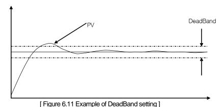
If setting deadband as in the figure, the PID control built in XGB may regard the error between PV and set value as 0 as long as PV is within the available scope of deadband from set value.
