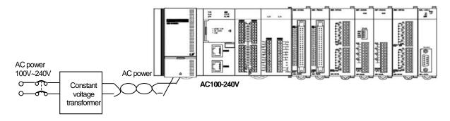
(2) Connect noise that include small noise between line and earth. (When there are much noise, connect insulated transformer.)
