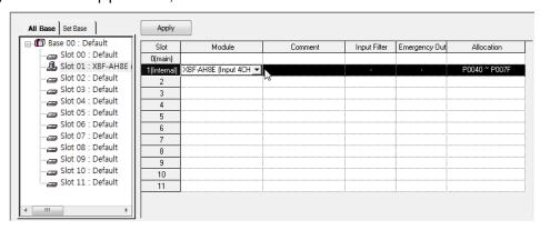
(6) A screen will be displayed for you to specify parameters for respective channels as below. Click a desired item to display parameters to set for respective items.
