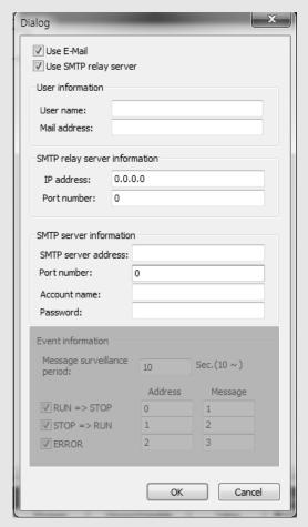
when selecting [Write] in XG5000 for communication parameter setting, PLC goes to stop to activate it, which falls under Event information. In this special case, service history would be missing
