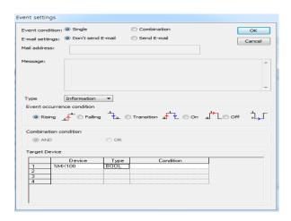
6) Select the timing of data saving at the Event Occurrence Condition. The number and timing of data change depending on the set value.
