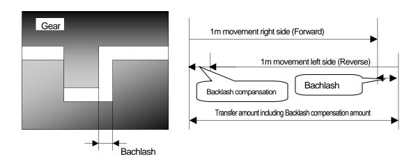
(e) It compensates by adding backlash compensation pulse to current output pulse within speed limit. In case backlash compensation amount is bigger than Max. output Pulse (Speed limit × Control cycle) for one control cycle, distribute compensation amount to several control cycles
