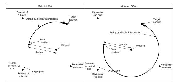
(c) If target position is same with start position, can progress circular interpolation. And the circle radius is distance from midpoint to starting position (=target position)
