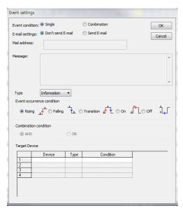
5) Select the condition setting menu to activate the following setting window. Select [BIT Condition], and input device values into the device window in BIT types.
