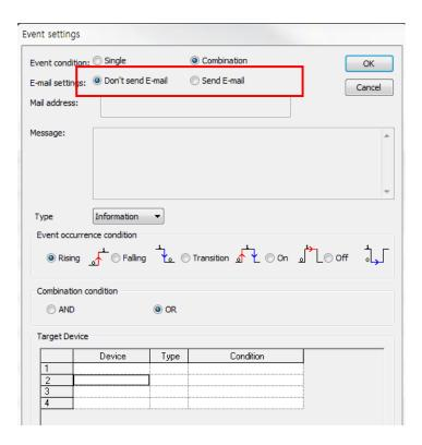
3) Select [Event Condition] and [Multiple Condition] to activate the condition setting window which allows for up to 4 inputs.
