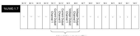
Interpolation output condition Bit On (1): Interpolation output
