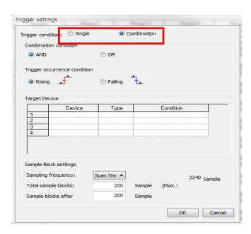
5) Select [Trigger Condition] and [Multiple Condition] to activate the condition setting window which allows for up to 4 inputs.
