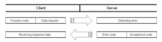
When receiving the abnormal frame from client, server transmits error code and exceptional code. Error code is function code adding 80(Hex) and exceptional code indicate the specific error content. Each code has following content.
