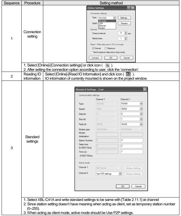
After standard settings, P2P channel and P2P block should be set. Setting methods are as follows.
