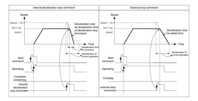
■ If the deceleration distance is longer than distance to target position when input deceleration stop command during positioning control operation, it will be stopped at the target position.
