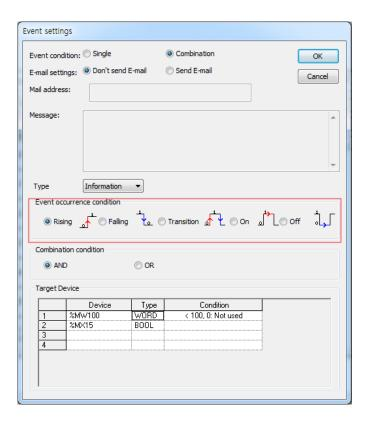
6) Select each condition setting menu one by one, inputting specific set values. [Multiple Condition] activates Event Condition by calculating [Single Conditions] using the set run method. The basic setting is performed in the same way as Single Condition.
