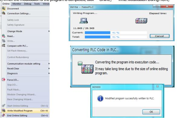
(6) When Write Program is completed, click <code>"Online"</code> - <code>"End Modification During RUN"</code> .
