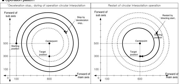
When decelerating in circular interpolation by dec. stop command and restart the same step no., not that executing circular interpolation after circular interpolation being executed 3 times, but that positioning at the goal position after going around 1 time, because 2 times of circular interpolation was executed in former operation.
