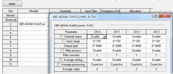
[Figure 6.20 A/D input mode setting window]
