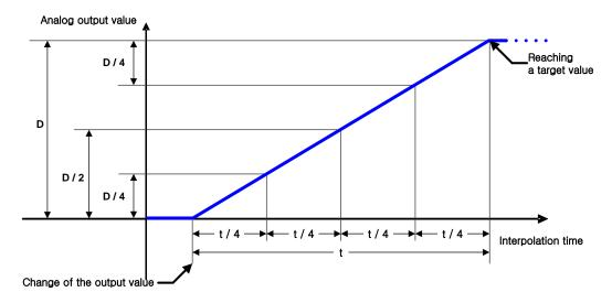
(3) S-type interpolation: The output is changed up to objective value with S-type during the interpolation time.
