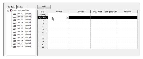
(4) Click the arrow button on the screen above to display the screen where an applicable module can be selected. Search and select the embedded analog input/output module to select.
