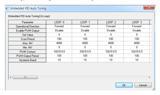
[Figure 6.18 Auto-tuning parameter setting window]
