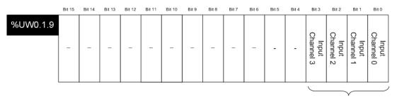
Minimum limit warning detection Bit On (1): occurrence of minimum warning Bit Off (0): Normal
