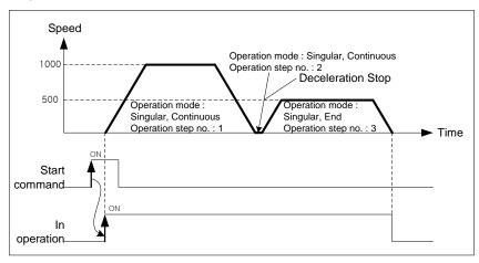
The Step1 will be operated by the start command. However, because the moving amount of next step is 0, it stops after deceleration, and then operates Step3 after 1 control period.
