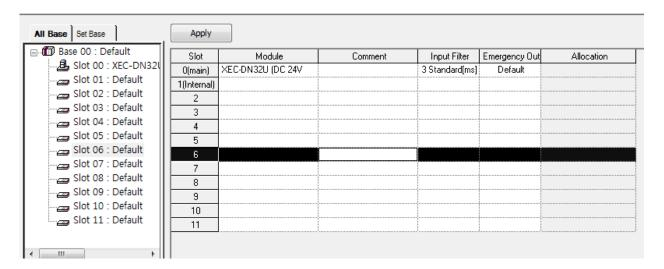
If you press "In Detail," button on the slot image or the relevant slot position in the base window as below, the window for setting the filter, emergency output will be displayed.
