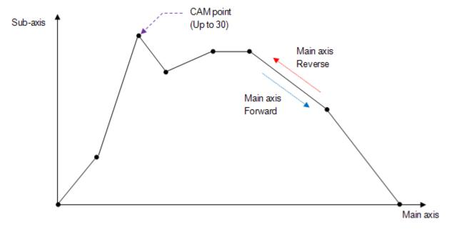
Like figure above, you can set up maximum 30 CAM data points, and it operates CAM curve between CAM points with straight line. CAM point data is set up at sub-axis and as type of (main-axis position, sub-axis position). CAM data point can be saved at the specified memory address of each axis by using "Write Variable Data" (XVWR, XPM\_VWR) command. For memory address to save CAM data point of each axis, refer to 3.10 User CAM data memory address.
