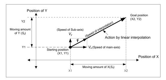
Speed of sub( $V_y$ ) = Speed of main ( $V_x$ ) ×  $\frac{\text{Moving amount of Sub}(S_y)}{\text{Moving amount of Main}(S_x)}$
