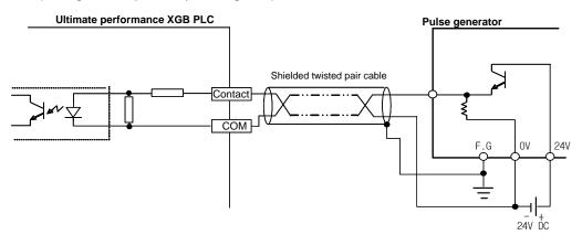
(2) When pulse generator is open-collector output type.
