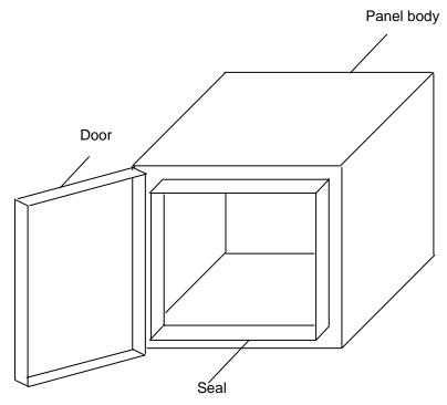
(e) To ensure good electrical contact with the control panel or base plate, mask painting and weld so that good surface contact can be made between the panel and plate.
