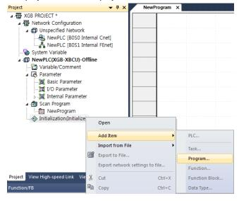
(b) The screen for registering the task will be displayed. Click "Fixed cycle" in the execution conditions and after entering the task name, input the items required for setting as below
