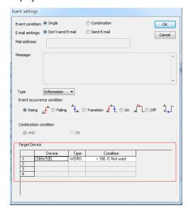
6) Select the timing of data saving at the Event Occurrence Condition. The number and timing of data change depending on the set value.
