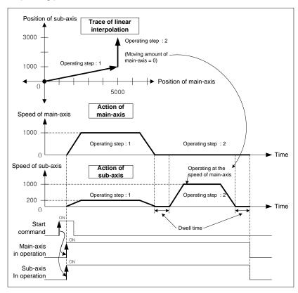
(4) 2 axes linear interpolating continuous operation with circular arc interpolation
