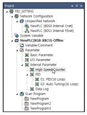
(b) Selecting high-speed counter opens a window to set high-speed counter parameters as follows. (Every parameter settings are saved in the special K device area.)
