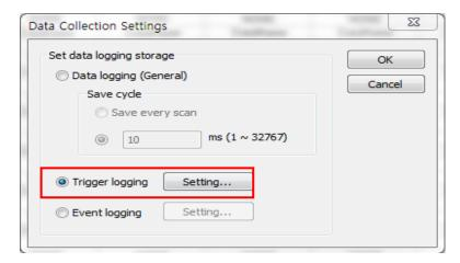
4) Upon selection, the following window is activated for trigger setting. Select [Single Condition] as the Trigger Condition. Select either [Elevation] or [Descent] as the Trigger Occurrence Condition.
