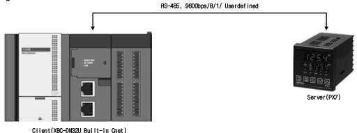
[Figure 2.11.3] User defined communication system configuration
