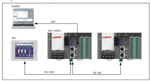
(3) Configuring 1:N communication system with the maximum 32 stations by using the basic unit's embedded RS-485port
