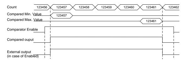
7) Mode 6 (Count value ≤ Min. set value of Compared Output 0 or Count value ≥ Max. set value of Compared Output 0) If present count value is less than or equal to the minimum set value of compared 0 and greater than or equal to the maximum set value of compared 0, output is sent out, and if count value increases/decreases to exceed compared value's range, output is not sent out.
