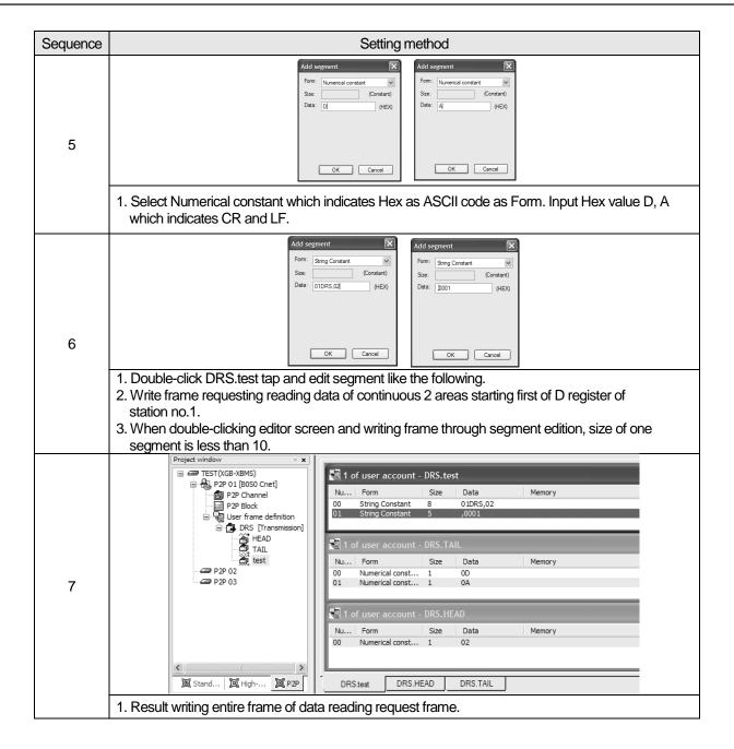
4) Writing frame to receive response frame of temperature controller
